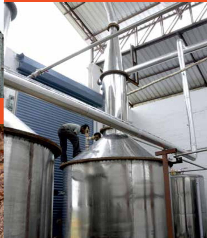
The pot stills for double distillation. Thereafter, it's storage and bottling.
