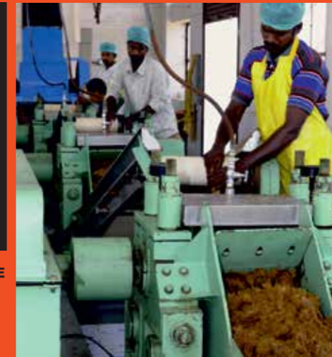
Shredded and put through presses to squeeze out the juice.
